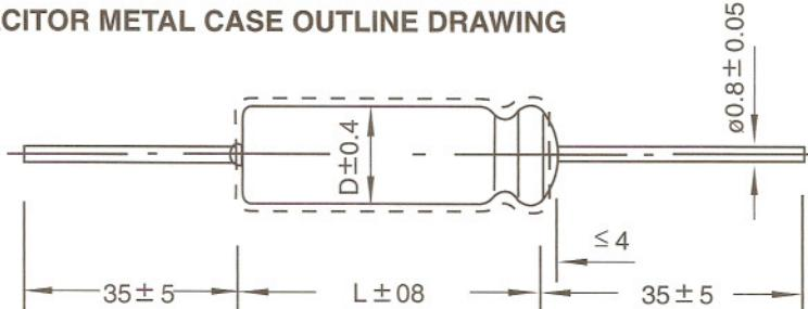
Dimensions Millimeters mm
